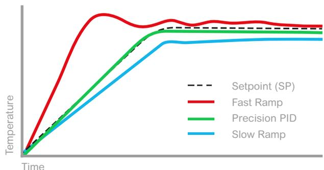
Ramp rate controls the rate of change to setpoint, keeping the material within specified temperature limits, minimizing damage and distortion in the final product. A holdback "Guaranteed Soak" function enables material to reach the required temperature before the process advances.
