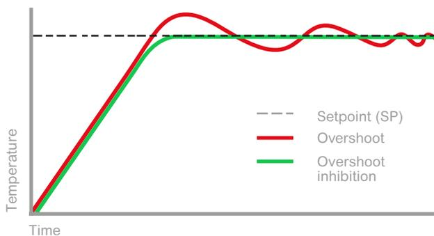
By automatically reducing power demand near the setpoint the Eurotherm cut back feature significantly minimizes overshoot which reduces waste and optimizes energy usage. This lowers the risk of parts not reaching operating temperature or overheating.
