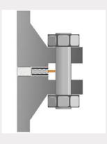
The FRG enables bolted joints to be easily and effectively sealed to prevent internal corrosion. The soft SIGMA inner ring of the FRGs conform seamlessly to the flange face, even if already damaged to:
