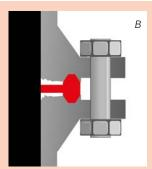
A: standard Octagonal RTJ - liquid can get in between flanges and cause erosion/ corrosion in this area.
