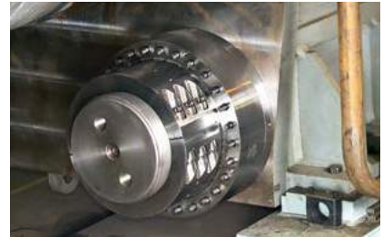
Split-Nut thrust collars are a custom designed product from Superbolt that are much easier to install and remove than other large threaded fasteners on large press columns.
