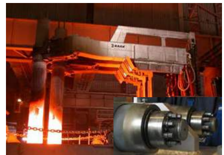
EAF electrode arm assembly. With the MJT, a high clamp load could be achieved to withstand the extreme vibration acting on the electrode arm.
