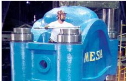
Eight Superbolt column nuts required only 12 man hours for installation vs. 2-1/2 full days for heating of columns.
