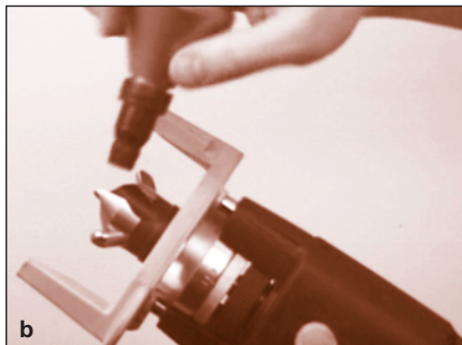
FIGURE 78 (a and b): Lubricating the drill head
