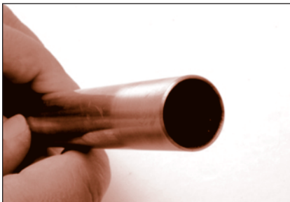
FIGURE 55: Properly prepared tube end
