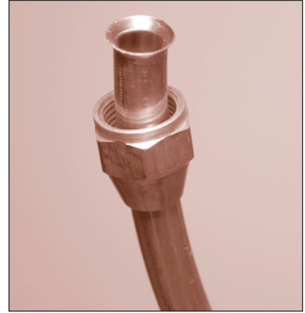
FIGURE 32: Completed flared tube end
