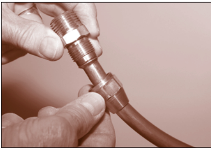
FIGURE 28: Flare fitting/flared joint during assembly
