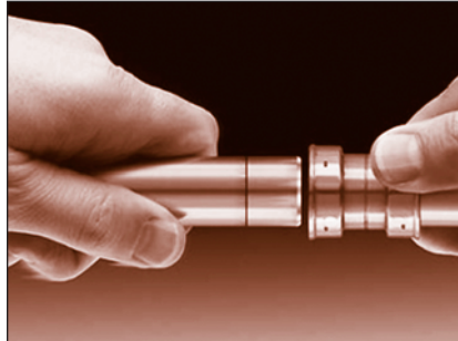
FIGURE 72: Aligning tube end squarely
