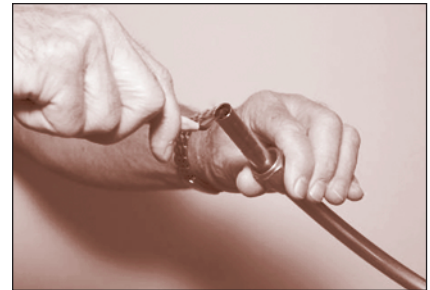
FIGURE 30: Reaming prior to flaring the tube end
