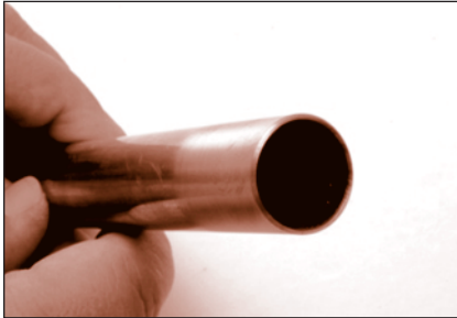
FIGURE 69: Chamfered tube end
