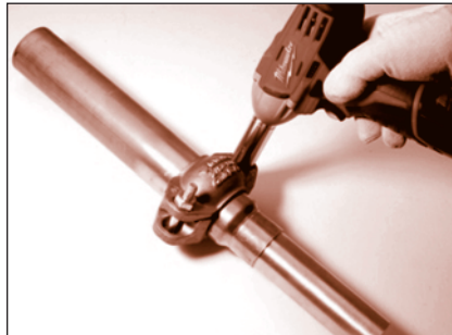
FIGURE 43: Tightening the clamp
