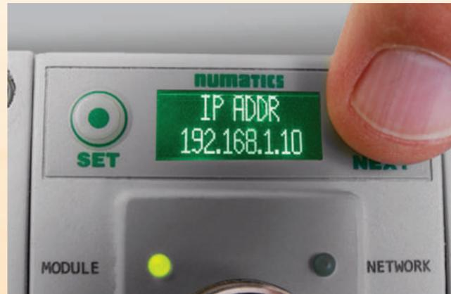
The G3 offers a high-speed, digital distributed solution allowing star or in-line topology, reducing the length of cable runs and pneumatic connections required and helping to lower costs and improve performance. It also provides a wide range of I/O capabilities, including analogue, digital (on/off) and temperature. This helps to make purchasing and engineering simpler as all options can be taken care of with a single device family.
